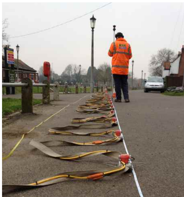
A series of geophones arranged along a MASW survey line
