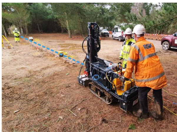
Deployment of tracked vibrating source.
