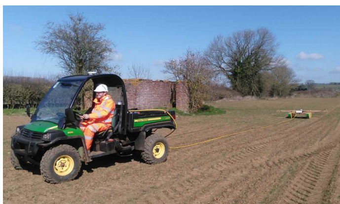
The CMD Explorer instrument shown above uses transmitter and receiver coils at either end of the boom. This version is a multi-depth sensor as the booms contain three pairs of coils at an increasing spacing.
