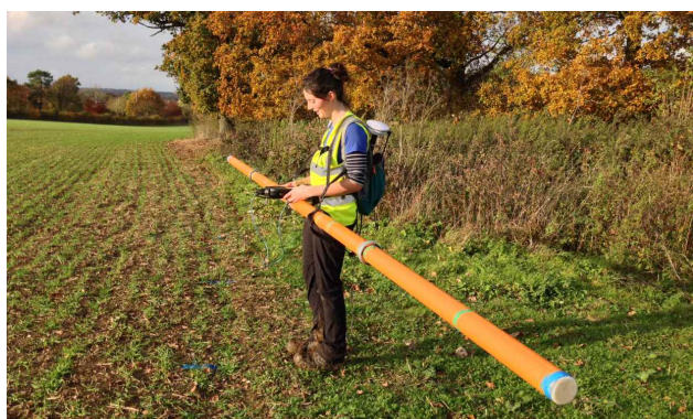
The CMD Explorer instrument shown above uses transmitter and receiver coils at either end of the boom. This version is a multi-depth sensor as the booms contain three pairs of coils at an increasing spacing.
