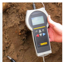
Deployment of VES equipment to test the soil resistivity to shallow depths to support a new substation installation
