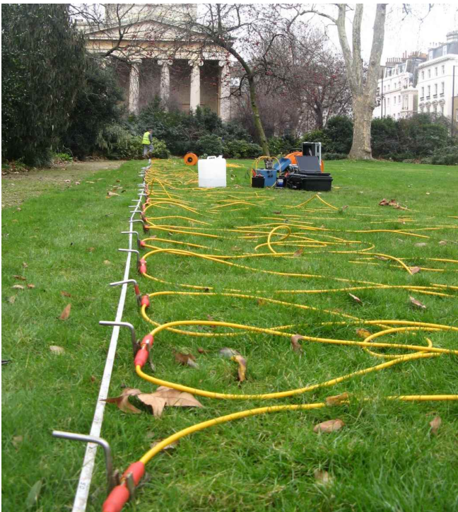
A typical electrical resistivity tomography survey comprises an array of electrodes placed along a line. The length of the line determines the depth penetration, and the electrode spacing determines the resolution.
