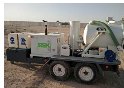
Hydro-vac excavation can be used to safely expose buried live utilities.
