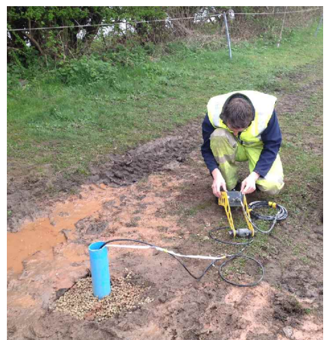
Acquisition of magnetic data down a borehole using a vertical gradient magnetometer probe.
