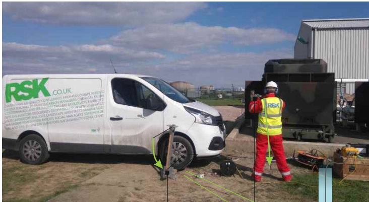
Above: The downhole set-up. Note the shear beam is typically weighted with a vehicle to prevent movement. First arrivals of the seismic wave trains from each receiver are picked to determine the velocities and dynamic moduli (see below )
