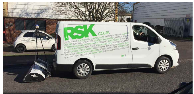
Vehicle mounted GPR systems can provide huge productivity benefits on highways with limited access
