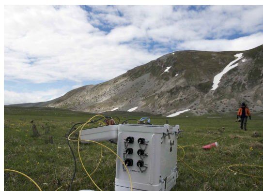
Deployment of electrical imaging equipment
