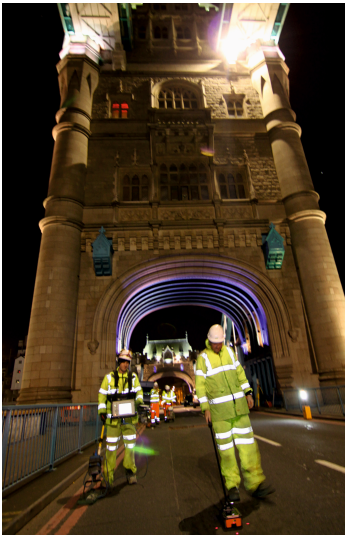
GPR can be used successfully to investigate listed buildings where minimal disturbance to the fabric of the structure is of paramount importance.
